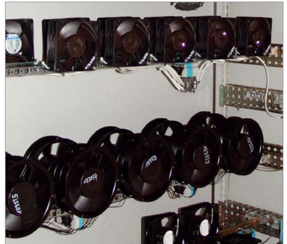
Figure 2: Test candidates in the test lab; they undergo the endurance test at 40 °C and 70 °C until they break down. (photo: ebm-papst)
