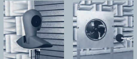
Room for precision noise measuring
