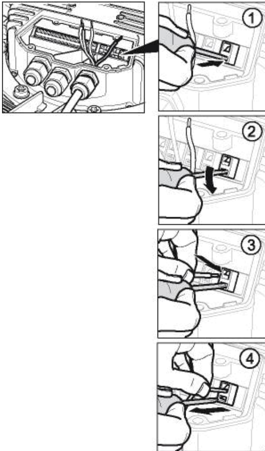
Fig. 2: Connecting wires to terminals
