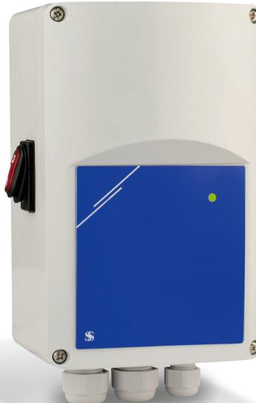
The EVS-1-XX-DM electronic speed controllers automatically control the speed of single-phase voltage controllable electric motors (230 VAC, 50 / 60 Hz). These units are equipped with Modbus RTU communication and provide a wide range of functionalities: remote control options, adjustable off level, min. and max. output voltage settings, and time-limited motor operation initiated by a logic or switch signal.
