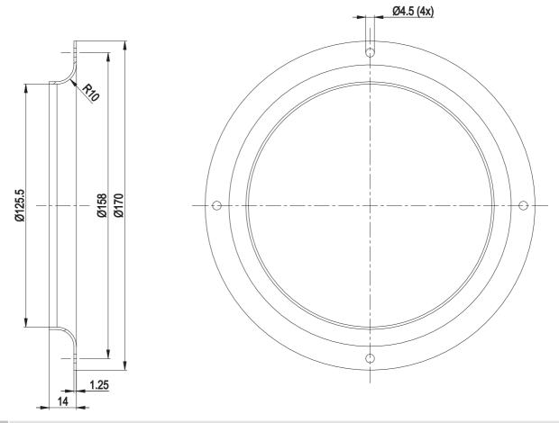
Accessory part: Inlet nozzle 09576-2-4013 not included in scope of delivery
